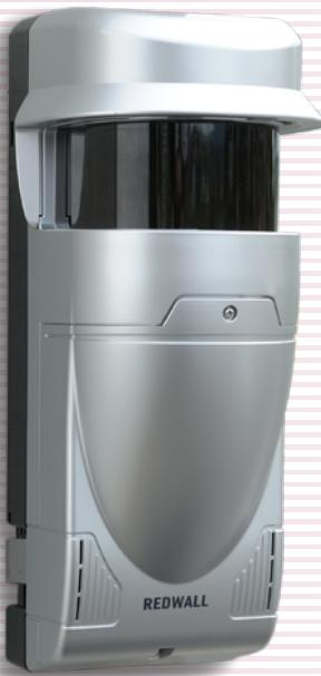
The REDSCAN RLS-3060 is an innovative laser scan detector. It can detect a moving object's size, speed, and distance from the detector and process that information with a unique algorithm, which results in hi-reliability detection of people with minimal false alarms.
